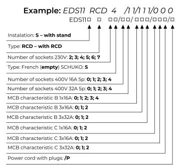
On request, it can be made with a 2m supply cable and a 16 or 32A 5p plug based on the switchboard rated current (variant /P).
