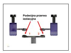
Fig. 3 Main connectors of LAS disconector
