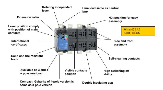
LA disconectors have very high durability, reliability, they are dependable and safe during usage, thanks to self-cleaning construction of double connectors and effective extinction chambers. Their functions and advantages are shown on Fig. 6. Quick, independent
